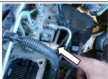
15. For 2019+ Models: Remove the fuel return line (1) by removing the fuel return line banjo bolts (2, 3, 4).
