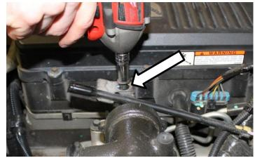
5. Loosen the clamp between the rubber coupler and the intake horn. Use a blade screwdriver to gently break the seal.
