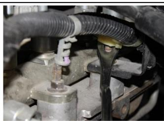
20. Disconnect CCV pressure sensor harness connector that is located at rear of the valve cover. This needs to be disconnected to allow you to coil the harness aside to access the grid heater.
