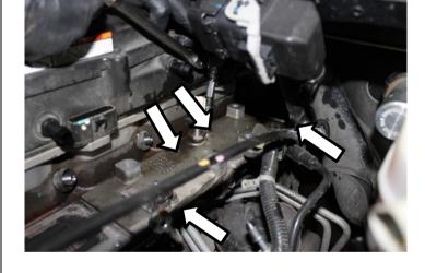
2. Reconnect the fuel rail connector. Then apply some pipe dope to the four OEM fuel rail bolts and install the fuel rail to the intake plate. Torque to 18 ft-lbs (24.4 Nm).
