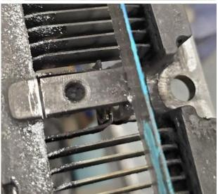
5. Install the nylon insulating washer to the bottom of the grid plate with the washer shoulder inserted into the bolt hole.
