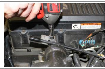
16. Reinstall the harness clip back onto the horn.
