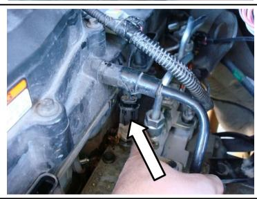
18. Disconnect the breather hose to the motor. Disconnect the two fuel line harness connectors on the side of the motor.
