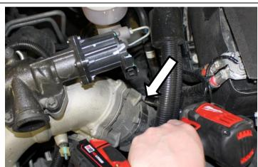
6. Pull off the harness clip from the intake horn.
