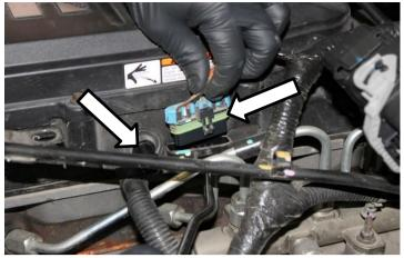
19. Using a puller tool pull out the harness clips that secure the harness to the grid heater and the other clip on the backside of the valve cover.
