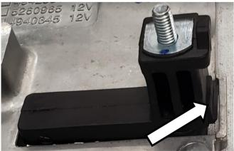
2. To remove the lower busbar, use the included IP25 Torx Plus bit and slim 10mm wrench to remove the bolt and nut in between the heating elements.
