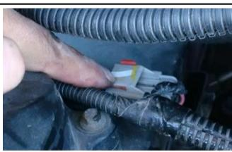
21. Disconnect the EGR servo motor connector.
