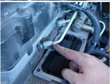
17. Disconnect the intake air temperature sensor connector from the grid heater.
