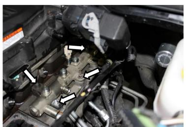
24. Disconnect the fuel rail connector from the back of the rail.
