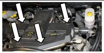
2. Disconnect the EGR valve connector from the EGR valve.
