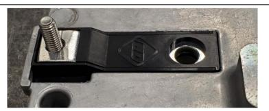
9. Install the M8 socket cap screw through the top into the lower busbar into the lower busbar. Torque to 15 ft-lbs (20.3 Nm).
