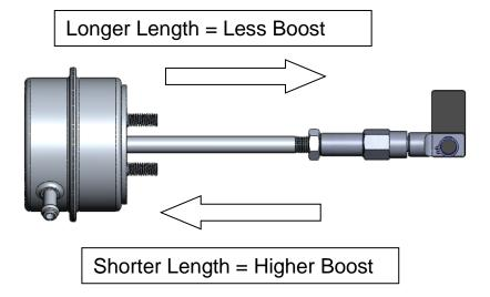
You can now easily adjust your boost pressure without removing the retaining ring.
