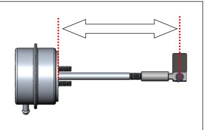
2. Then you will need to apply regulated shop air (<50psi) to the wastegate diaphragm to release the tension on the wastegate rod.
