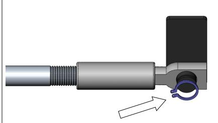
4. You can now un-thread the rod end from the shaft. Note that you will need to release the jam nut if there is one.
