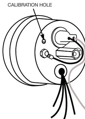
**IMPORTANT:** This Tachometer has a new, improved meter movement. The tach pointer may not rest at zero with engine off. This is normal. When engine is started the pointer will position on the correct rpm.
