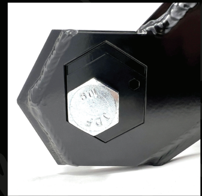
Highest caster setting +6° (5"-6" Lift with no drop bracket)
