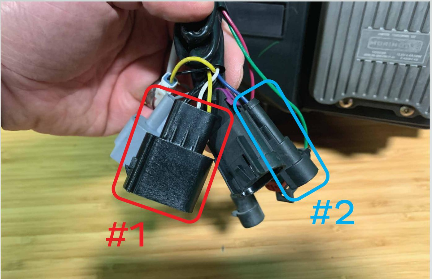
3. Get the supplied adaptor harness and plug in these 2 connectors into the harness on the back of your XB headlight.
