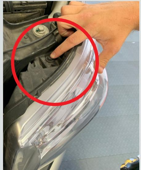
4. Remove the headlight and unplug the factory bulbs from each socket.
