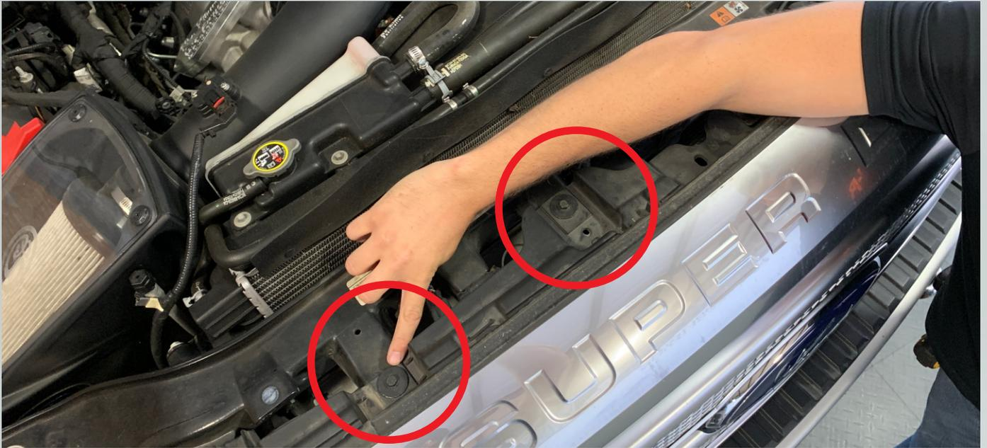
2. Use a long flat-head screwdriver to depress the five clips at the bottom of the grille shell to release it.
