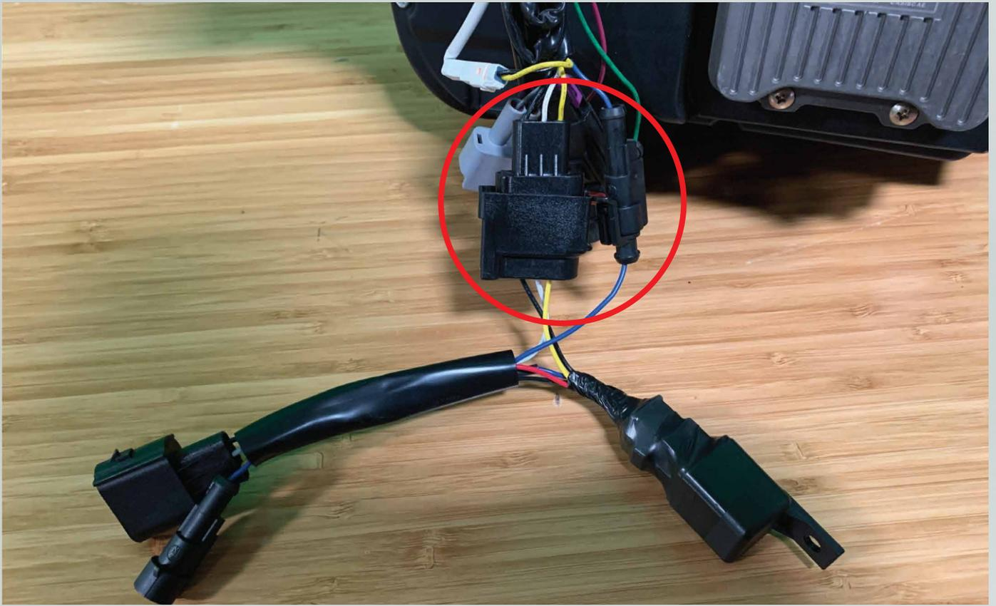
3. Plug these connectors (#1) into the truck harness and mount the relay (#2) to secure it.
