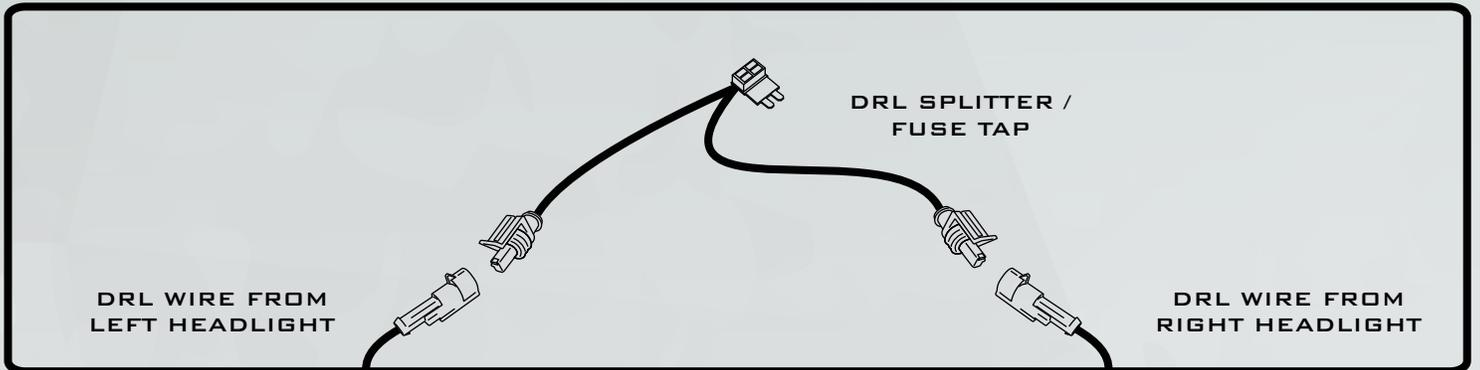
6. Connect fuse tap to the power mirror fuse (#50) indicated below:
