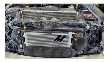
**16.** The bottom of the plastic mount will need to be trimmed to install the remaining Mishimoto transmission line. Position the line in place to mark where the mount will need to be trimmed.
