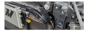
**20.** Using a 13mm socket, remove the upper fan shroud bolt and install the supplied line bracket in this location. Attach the supplied p-clip to the upper factory transmission line and secure it to the line bracket with the supplied M5 bolt and lock nut.
