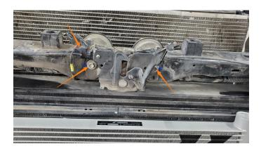
12. Drill a ¾" hole through the shroud on the mark that was made in Step 10. Then, reinstall the shroud and hood latch. Check that the hood closes and latches properly. Adjust the position of the hood latch if necessary.
