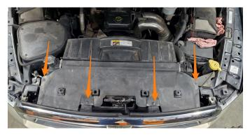
2. Using a 10mm socket, remove the four (4) bolts securing the grille to the frame. Then, remove the grille from the vehicle by pulling the bottom of the grille straight out.
