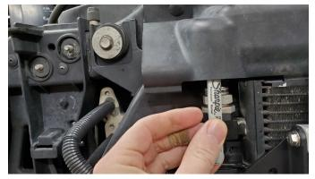
11. After making the mark, remove the shroud from the vehicle to be drilled by removing the plug from the hood latch. Then, using a 10mm socket, remove the two (2) bolts securing the hood latch to the frame so the shroud can be slid off the hood release cable. Marking the position of the latch on the frame before removing it will help to reinstall it in the correct position. (Image on next page)
