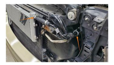
10. Position the plastic shroud that was slid out of the way in Step 3 back into place. Then, make a mark on the shroud directly above the fitting on the passenger-side of the stock transmission cooler.
