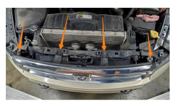
3. Remove the hood release cable from the plastic clip, remove the two (2) trim clips securing the plastic shroud to the frame, and slide the shroud out of the way.
