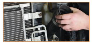
7. Mark the transmission cooler hoses. It's recommended that the mark be five inches back from the hump. Once done, cut the hoses on your mark.
