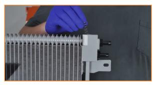
24. Lower your bypass plug into the recess opening.25. Position the black aluminum piece at the top of the bypass plug.
