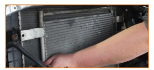
Install the stainless-steel hose barbs provided in your kit to the transmission cooler hoses. (2x worm gear clamps)
