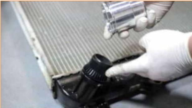
3. Install the Mishimoto lower coolant hose by feeding the hose through the engine bay from underneath the truck. Secure the hose with two 2.75" T-bolt clamps on the larger ends. Use the factory clamps for the two ancillary lines. Once the hose is properly positioned, tighten all clamps.
