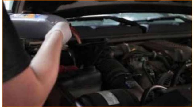
7. Start the vehicle and set the heat to high to purge the cooling system of any air bubbles. Allow the vehicle to reach operating temperature and check for any leaks.
