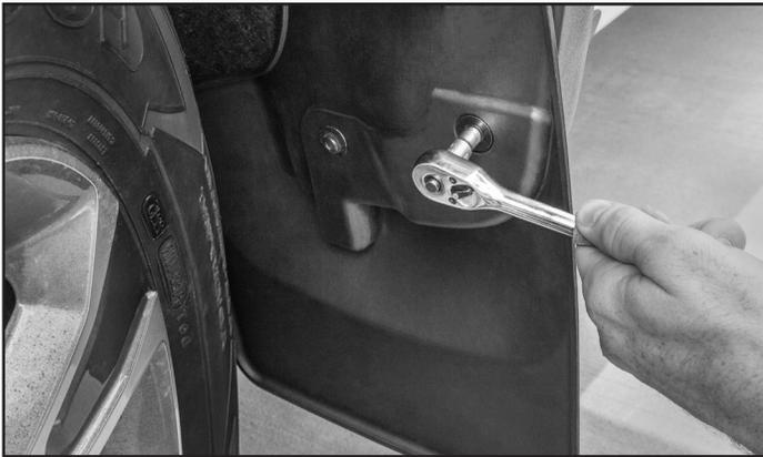
**9** Install the provided screw with the washer into the center hole and tighten.
