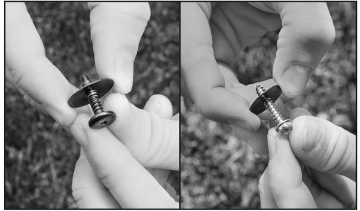
**8** Remove the washer from the remaining factory fastener and install on the provided hex head sheet metal screw.
