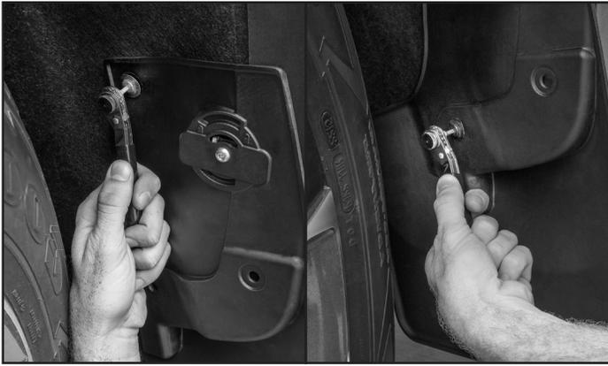
**7** Using the (2) previously removed factory screws, thread them through the top and bottom holes in the MudFlap and tighten.
