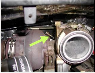
16. Position and install turbine inlet v-band clamp and torque to 110-130 lb-in.
