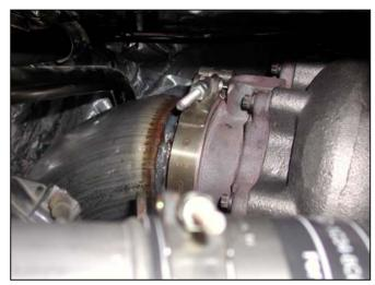
17. Install downpipe. Guide the v-band flange to mate with the turbine discharge flange. Install v-band clamp & torque to 110-130 lb-in.
