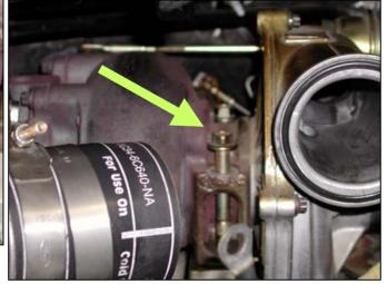
15. Install and tighten 2 turbo "hold down" bolts and torque to 35-37 lb-ft..
