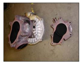
11. Remove the backpressure valve assy from the old turbo and install on the new turbo. Use anti-seize compound on the threads & torque the bolts to 185 - 215 lb-in.
