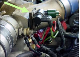
2. Remove the boost control module from the front of the x-section pipe
