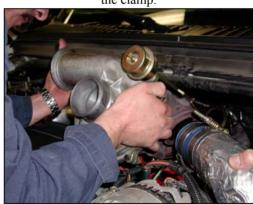
10. Make note of the turbo's position and how it fits on the engine for future reference. Lift the turbo off the pedestal and remove from the vehicle.
