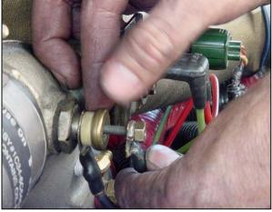
3. Remove the temperature sensor wires from the front of the x-section pipe
