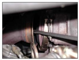
6. Using a 7/16" deep socket, loosen turbine outlet v-band clamp and move clamp off of the flange. Separate down-pipe from turbo
