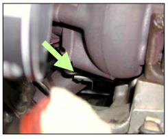
8. Reach under turbo and slide the clip on the EBPD control rod towards the pedestal to free the EBPD crank
