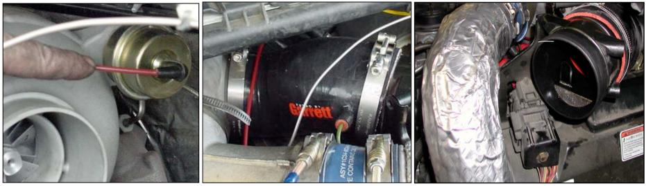
20. Re-install the red wastegate hose onto the wastegate hose actuator
