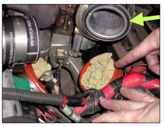
18. Remove covers (rags in this picture) from the intake manifold openings. Re-use the original compressor discharge O-ring and mount it into the new compressor discharge groove. A light coating of RTV or grease can be used to hold it in place.
