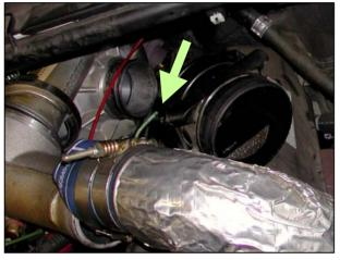
Before beginning, be sure to disconnect the negative terminal of the battery. 1. Unplug the green hose from the compressor intake duct. Remove the intake duct and crankcase breather
