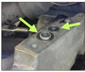
12. Ensure the 2 supplied o-ring oil seals are properly seated on the pedestal.. The turbo oil drain hole will pilot on the raised sleeve.
