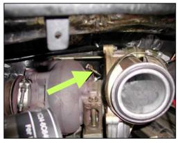
7. Using a 7/16" deep socket, loosen turbine inlet v-band clamp & move the clamp off the flange. This is the most difficult step of the installation. Use penetrating oil to help loosen
