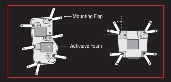
Rotate the mounting flaps on the rear side of the racing pedals, adjust each flap to a proper angle against the vertical/horizontal line, corresponding to the shape and the size of the factory pedal.
