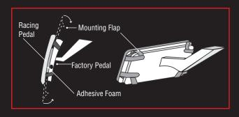
2. To install on the smaller size pedals, keep extra flaps not needed in their fold-in positions (Fig. 2)
