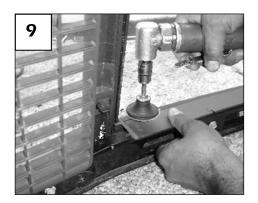
Make additional cuts to finish the required cut edge (8). Use a sanding disc or file to smooth and blend the cuts in each corner (9).
