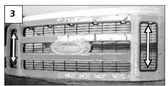
The OE black plastic inserts secured to the side openings (3) must be retained for installation.
