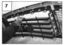
The OE black plastic inserts secured to the side openings (3) must be retained for installation.
