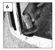
Test fit the center insert behind the OE grille; the ends of the billet bars rest behind the cut edge. Remove any additional material that must be trimmed for installation (4). When completed; the billet will rest flush behind the OE grille opening.
