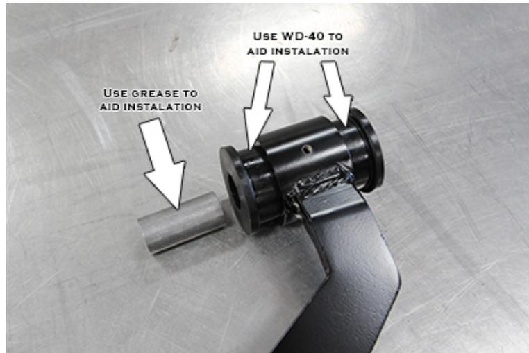
**Figure 2: bushing and crush sleeve installation**
