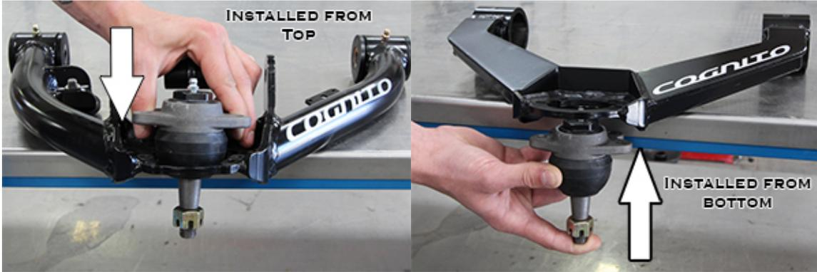
**Figure 1: ball joint installation**
