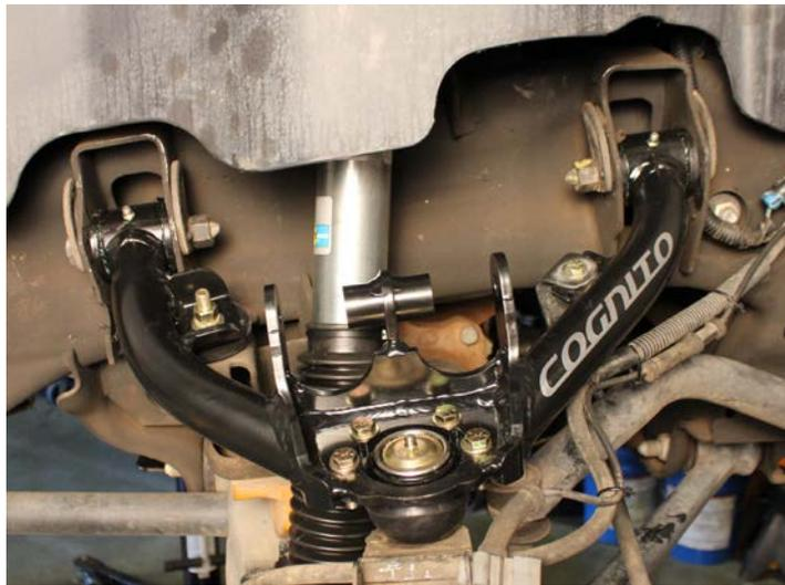
**Figure 3 Passenger side Cognito control arm installed**
