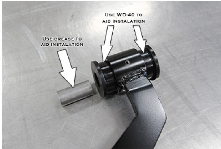
Figure 3: bushing and crush sleeve installation
