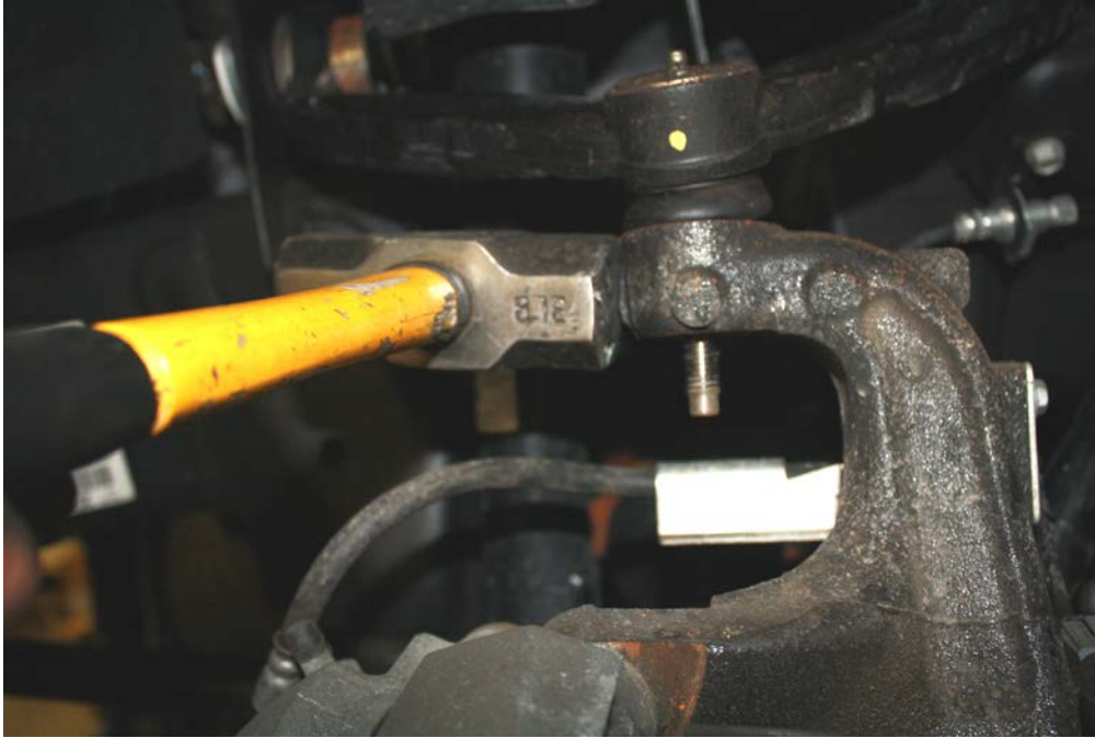
Figure 1: breaking ball joint loose from spindle
