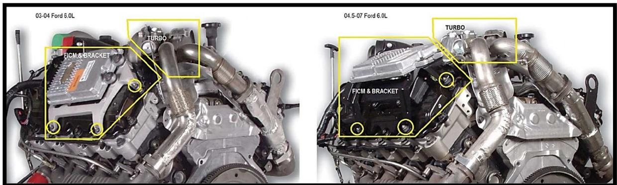
2. Remove the V-band clamp joining the factory y-pipe assembly to the turbocharger turbine inlet. (Save for reinstallation)
