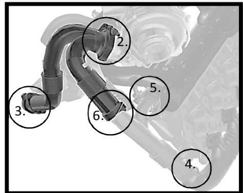
5. Remove the v-band clamp joining the passenger side up-pipe to the EGR cooler.
