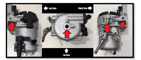
**Step 8:** Remove the bolts securing the fuel filter housing to the engine and remove the housing.
