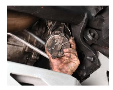
Clean all hardware in preparation to reinstall your new XDP Wrinkle Black HD Gear Reduction Starter. We do suggest using low grade Loctite (blue).
