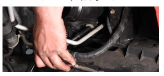
While tilting radiator towards engine pull up on right side of rad and twist out. (Figure 8)
