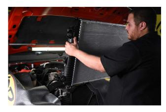
Install your new XDP X-TRA Cool Direct-Fit Replacement Radiator in reverse steps of removing your OEM radiator. (Figure 9)
