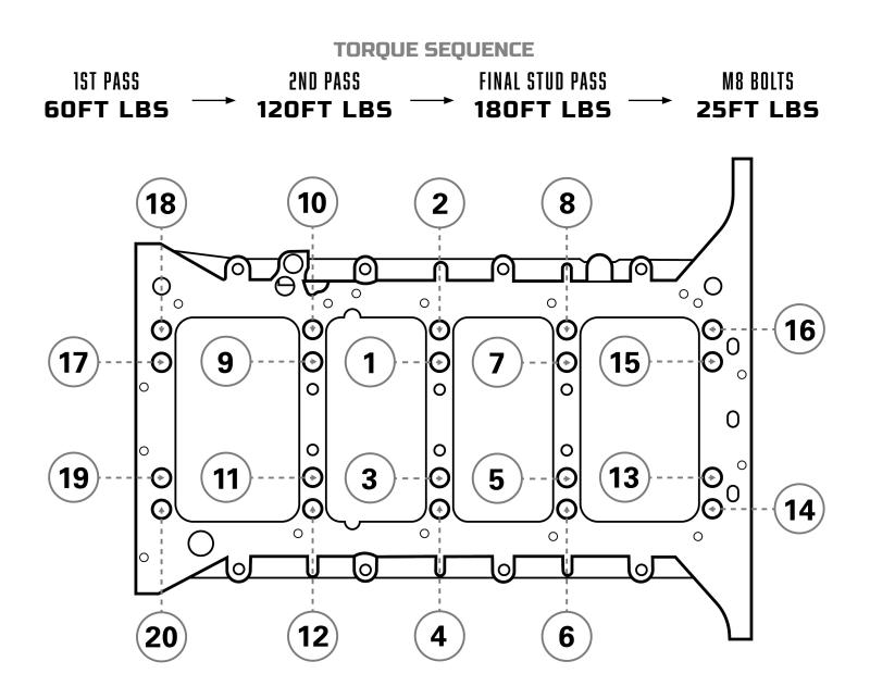
**NOTE**: After installation it is required to inspect the main bearing bores for proper size, and any out of round conditions as clamping force and tolerances will change. If necessary, align hone the engine block. Main bores should be align honed using the same fasteners and lubricant that is being used during final assembly. Modification to the oil pan adapter may be required. Check the top of the main studs for proper clearance and modify the adapter if necessary.
