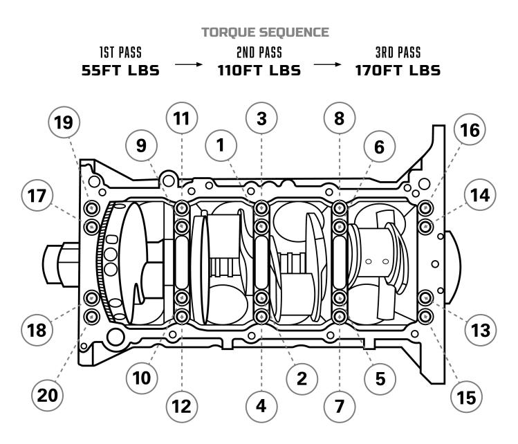
**NOTE**: After installation it is required to inspect the main bearing bores for proper size, and any out of round conditions as clamping force and tolerances will change. If necessary, align hone the engine block. Main bores should be align honed using the same fasteners and lubricant that is being used during final assembly.
