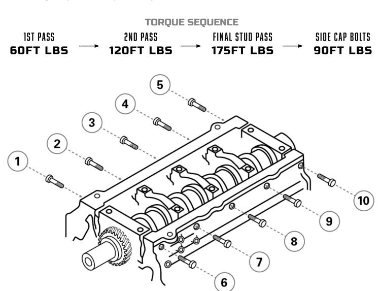
**NOTE**: After installation it is required to inspect the main bearing bores for proper size, and any out of round conditions as clamping force and tolerances will change. If necessary align hone the engine block. Main bores should be align honed using the same fasteners and lubricant that is being used during final assembly.
