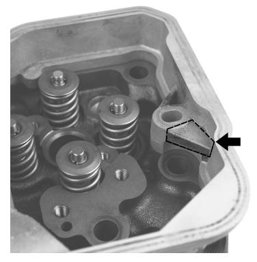
Following the torque sequence below in three steps, tighten the nuts to 40ft lbs, 80ft lbs, and then 125ft lbs.
