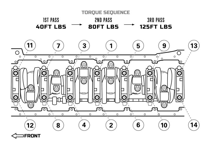
**NOTE**: After installation it is required to inspect the main bearing bores for proper size, and any out of round conditions as clamping force and tolerances will change. If necessary, align hone the engine block. Main bores should be align honed using the same fasteners and lubricant that is being used during final assembly. Modification to the oil pan adapter may be required. Check the top of the main studs for proper clearance and modify the adapter if necessary.
