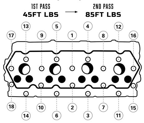
10 Following the torque sequence below tighten the nuts to 125ft lbs.
