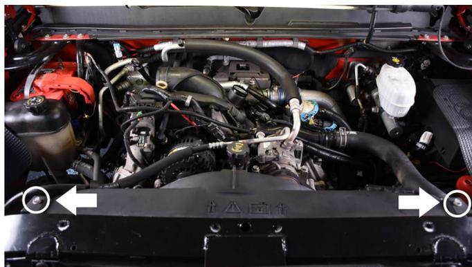
**4** Remove one push pin for the TCM and 4 push pins that hold the upper and lower shroud together. Once unclipped pull upwards and set aside.
