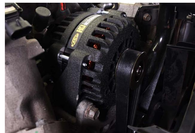
**Tech Tip-** For ease of new alternator installation lubricate the stainless steel bushings in the mounting ears of alt bracket.
