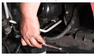
While tilting radiator towards engine, pull up on the right side of the radiator and twist out. (Figure 9)
