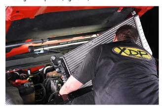
Install your new XDP X-TRA Cool Direct-Fit HD Intercooler, followed by reinstalling all other removed parts in reverse order. (Figure 12)
