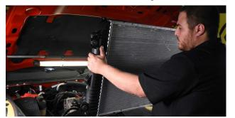
Remove the two bolts that secure the intercooler to the radiator support using a 13mm wrench or socket. (Figure 10)
