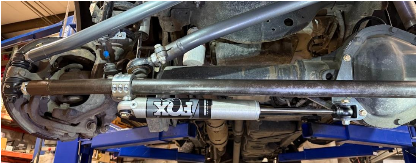
Figure 9. Correctly Installed Fox 2.0 IFP Stabilizer With The Steering Turned Passenger.
