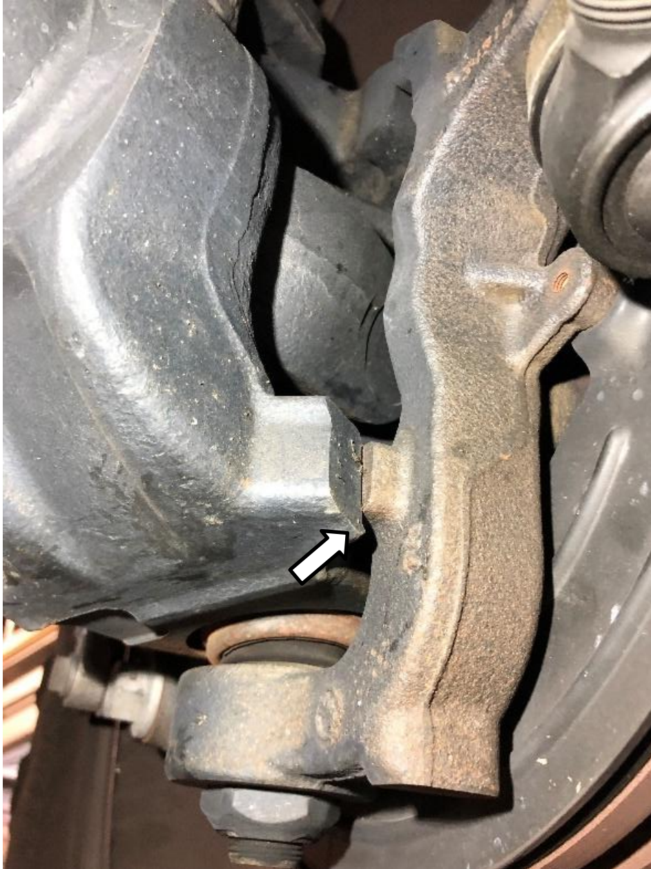
Figure 4. Driver Side Knuckle Fully Turned to the Passenger Side, Contacting the Steering Stop
