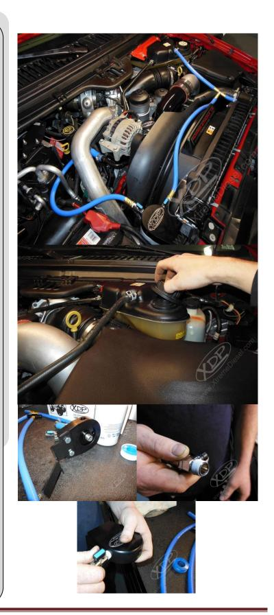
step 3: The XDP filter base will be mounted through a stud on the left of the radiator. Find the plastic battery cable retaining clip that is slid over a 10MM stud. This must be removed prior to mounting the bracket. The Mount has a long slender portion which should go between an opening in the plastic intercooler mounting bracket.
