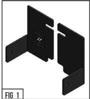
1) Begin by taking the ZROADZ Brackets and note where the ZROADZ Bracket mounting slots are located and that they will mount on the backside of front bumper.
